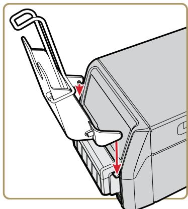
Use this tray only with the cutter accessory for the PD Series printers.
